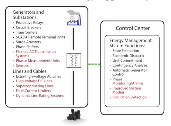
Note: Existing technologies and functions are listed in black; new and emerging elements are shown in red. SCADA = Supervisory control and data acquisition.
