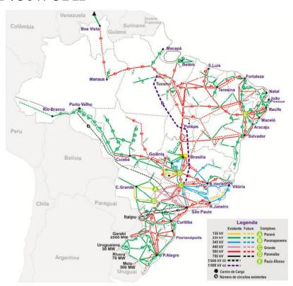
The Basic Brazilian Transmission System is composed of voltage lines in the range of 230kV up to 750kV.
