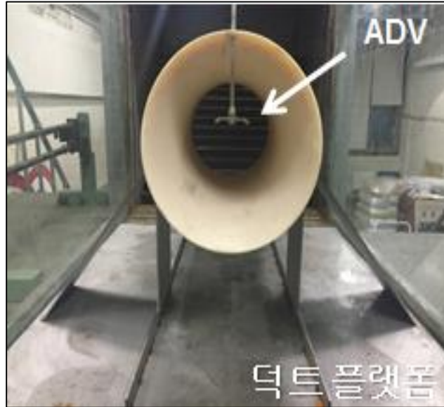
Fig. 8. Installed duct mock-up
