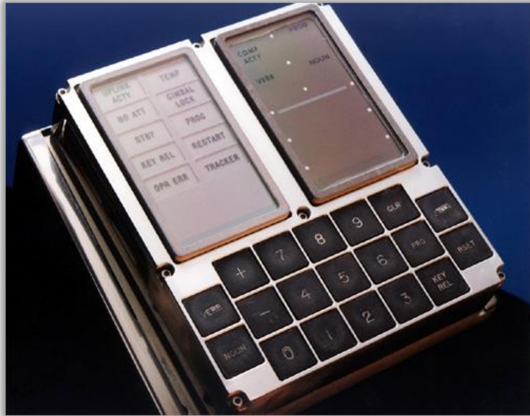
Apollo Guidance Computer, 0.043MHz clock speed. Image: NASA
